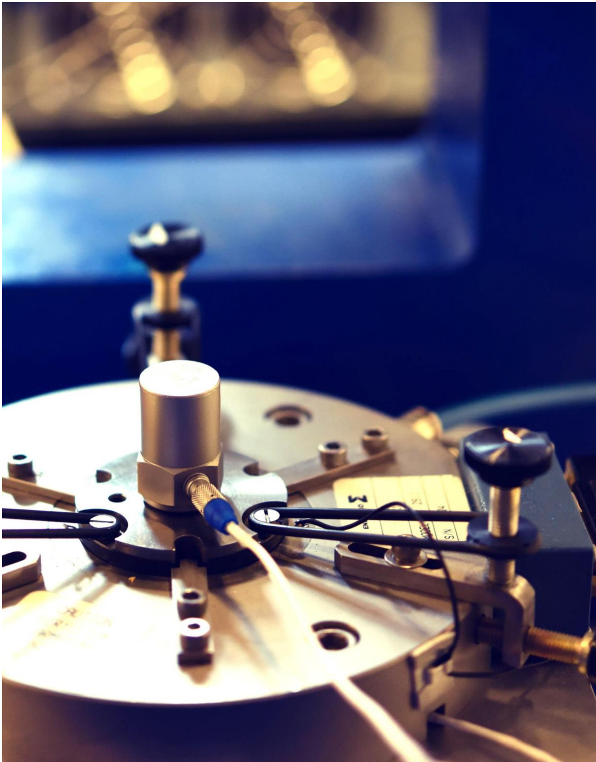
Photo no. 2 Mechanical vibration exciter – national measurement standard of mechanical vibrations
