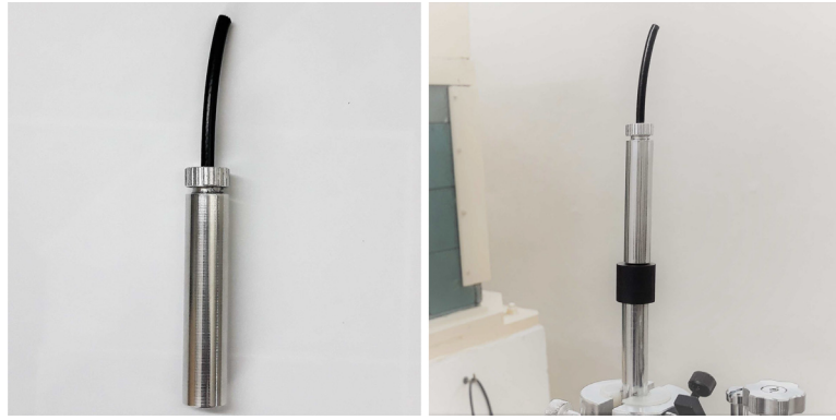
Fig. 10. Experimental setup for stem effect measurements: the dummy stem (left) and the prototype chamber with dummy stem on (right).
