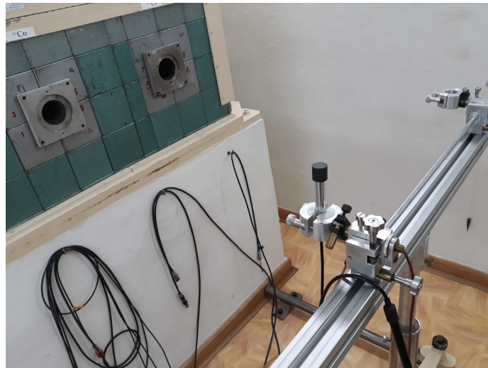
Fig. 1. The prototype ionization chamber type IGNAS-IC16A#001 in the test facility.
