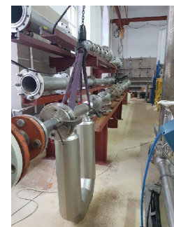
Calibration of Coriolis flow meter
