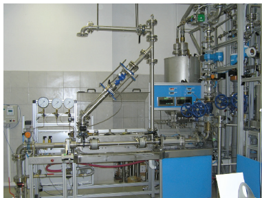
Reference standard of water volume flow and volume flow rate – testing of water meter in the 45-degree position
