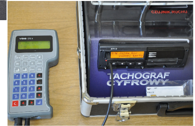
Digital tachograph in the training version and a device for its calibration and checking
