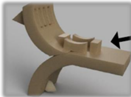
Fig. 3 - Visualize the free vibration of the cantilever. The deflection value is determined by a vibrometer, while the detector signal is measured by a proprietary electronic system.
