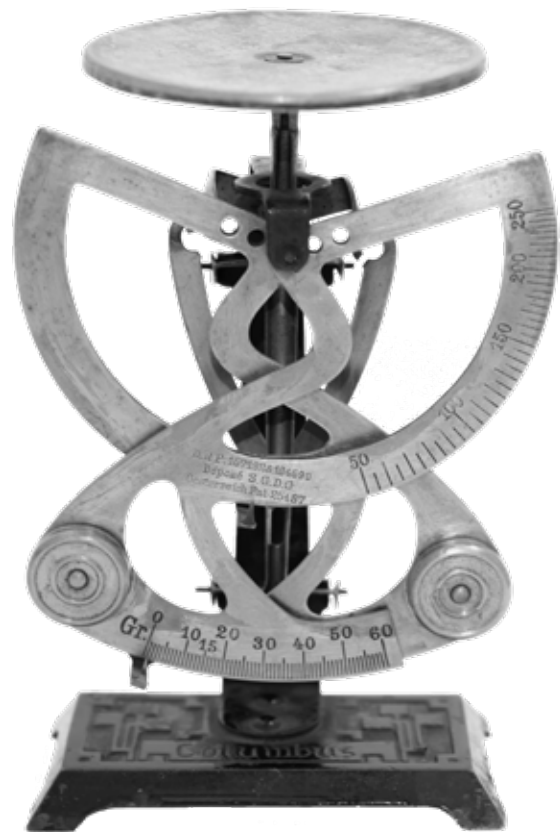
Two-lever letter scale, maximum capacity of 60 g and 250 g - ca. 1906-1919, cast iron, brass, manufacturer: Columbus
