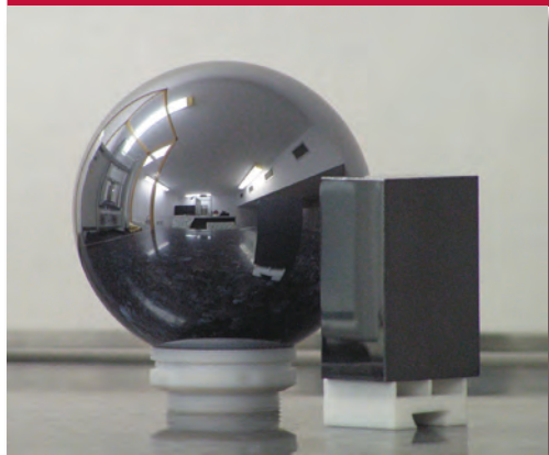
Density standards, made from single-crystal silicon: SILO2 sphere and WASO 9.2 rectangular prism
