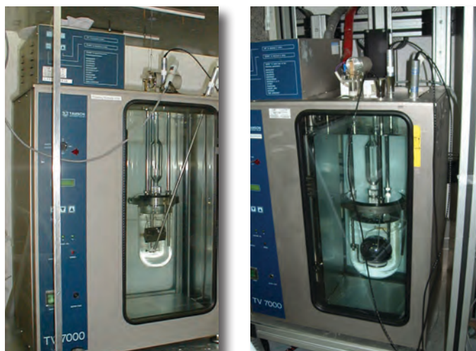
WASO 9.2 standard (on the right) and SILO 2 standard (on the left) while hydrostatic weighing, on their supports in the vessels immersed in the thermostats
