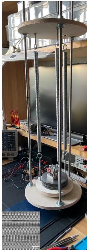
Figure 13. The Scanning Tunneling Microscope configuration. The STM scan head with vibration isolation system with background electronics. The acquired image of the HOPG atomic structure in the left corner [1].
